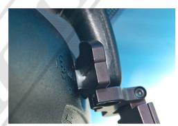
4 - Rotate the mount so it is parallel with the bottom of the mirror. Tighten the clamp screw untill the mount is securely attached to the mirror stem.
