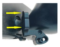
3 - When the mount is positioned as far forrward as it will go, tighten the clamp screw untill the Top and Mid Sections are slightly snug around the mirror stem. You should still be able to rotate the mount.
